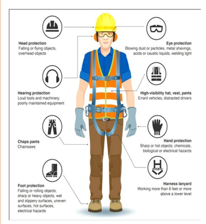
Fig. 5.1: The usage of personal protective equipment
