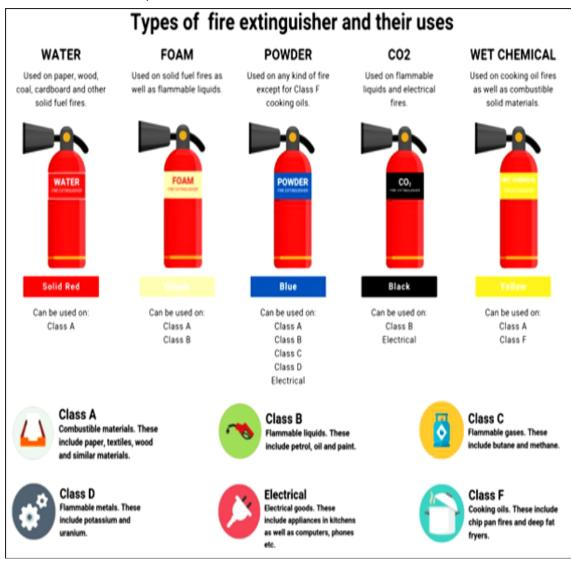
Fig. 5.2: Types of fire extinguishers
